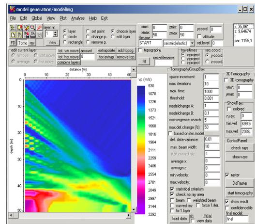
4. Control the tomographic result by a forward raytracing. For that purpose activate the option **ray**. The raytracing menu opens in addition.
