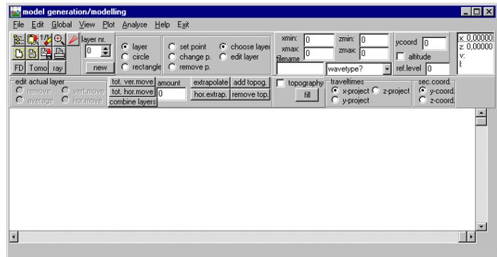
2. Choose the **wavetype** (e.g. electromagnetic for a GPR-modelling or acoustic for a raytracing).
