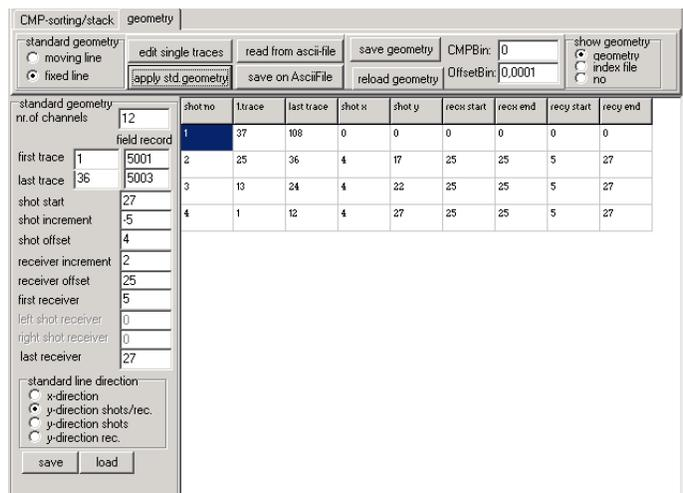
The parameters for the **borehole/surface** configuration (layout 3 of chap. IV.1.1 with 12 receivers within the borehole) are the following:
