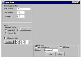
If you want to use a **velocity file** for the time-depth conversion instead of the **mean velocity** stored with each pick file first you must create such a velocity file (see section III). Then you must activate the option velocity file and load the wanted velocity file. The option **interpolate layer** controls how the special case of broken reflectors are handled (see below).
