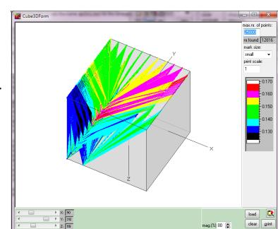
New option **restrict to max. angle °**. If activated only the pick data with an incidence angle smaller than the given one will be considered.
