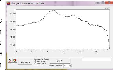
**smooth rec. xy-coord.:** option has been improved and after having completed the smoothing the original and the smoothed coordinates will be displayed for a direct check.
