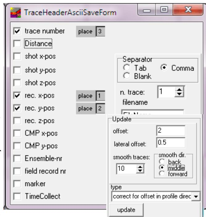
**Correct for offset in profile direction:** now the smooth directions can be entered. The possibilities back, middle and forward allow to simulate different coupling mechanism of GPS and source/receiver devices. Back might be useful for a flexible connection, middle or forward for a rigid one.
