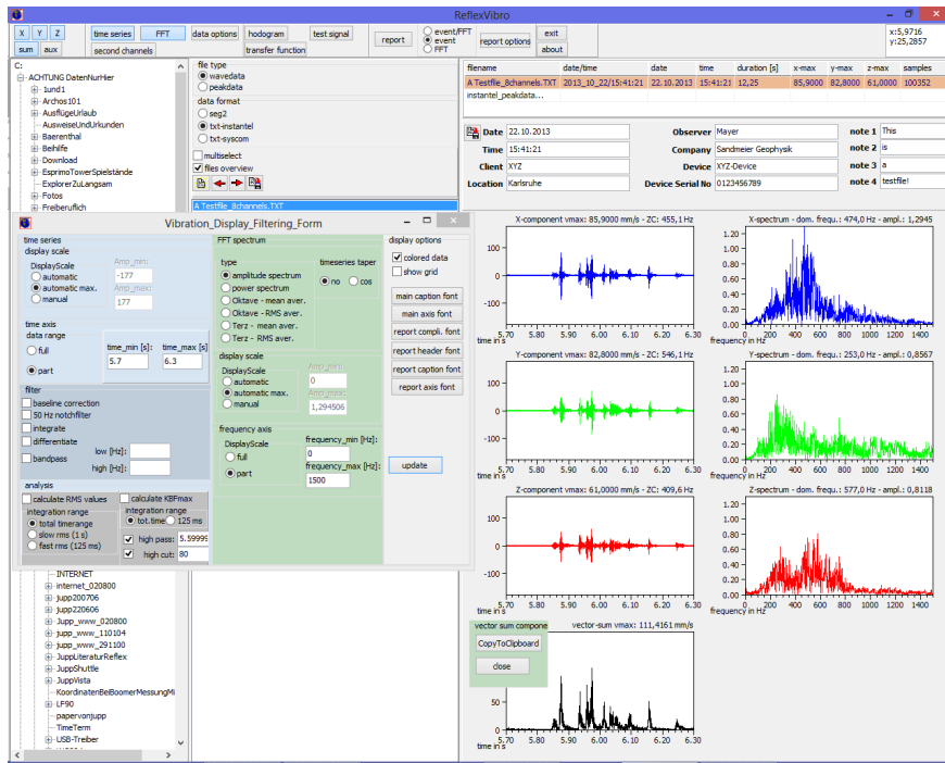
8-channel wave data set displayed with the indicated display and filtering options.
